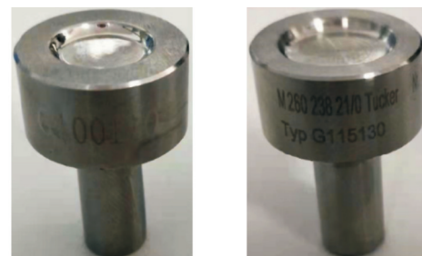
(a) G100110底模型腔深度1.1 mm (b) G115130底模型腔深度1.3 mm
